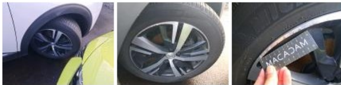
Jante alum. AVD bi-ton/polychrome, Griffe(s), E - Remplacer
